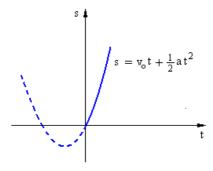
$$s = \frac{1}{2}(at + 2v_0)t = \frac{1}{2}at^2 + v_0t$$
