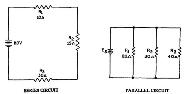
Figure 1-38. Series and Parallel Connected Resistors.
