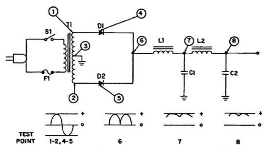
Figure 1-15. Simple Power Supply (Schematic).
