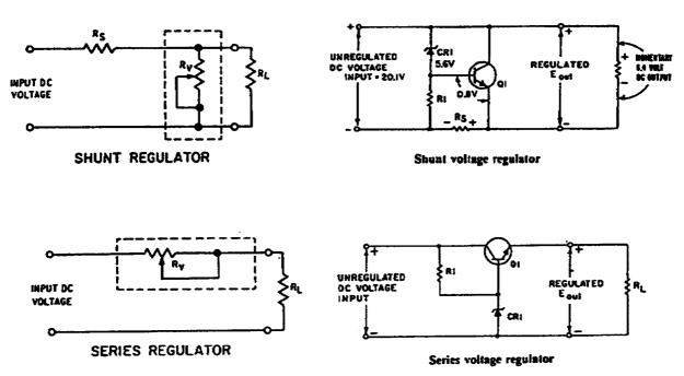
Figure 1-42. Regulator Circuits.
