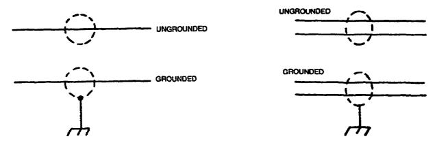
Figure 1-2. Shielded Conductors.
