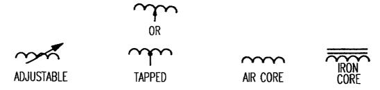
Figure 1-10. Special Purpose Inductors.
