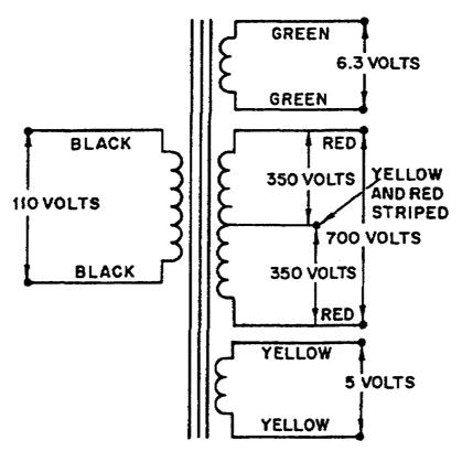
Figure 1-40. Power Transformer.
