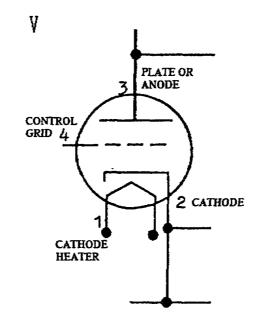
Figure 1-24. Triode Vacuum Tube.
