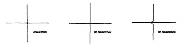
Figure 1-1. Crossing Conductors.
