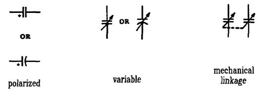
Figure 1-8. Special Purpose Capacitors.
