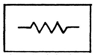
Figure 1-3. Fixed Resistors.
