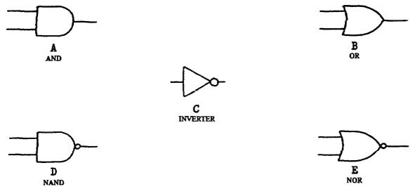
Figure 1-31. Logic Circuit Gates.
