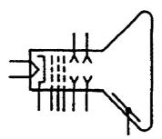
Figure 1-27. Cathode-Ray Tube (CRT)
