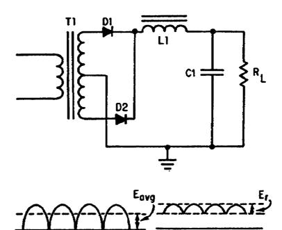
Figure 1-39. Filter Circuit.
